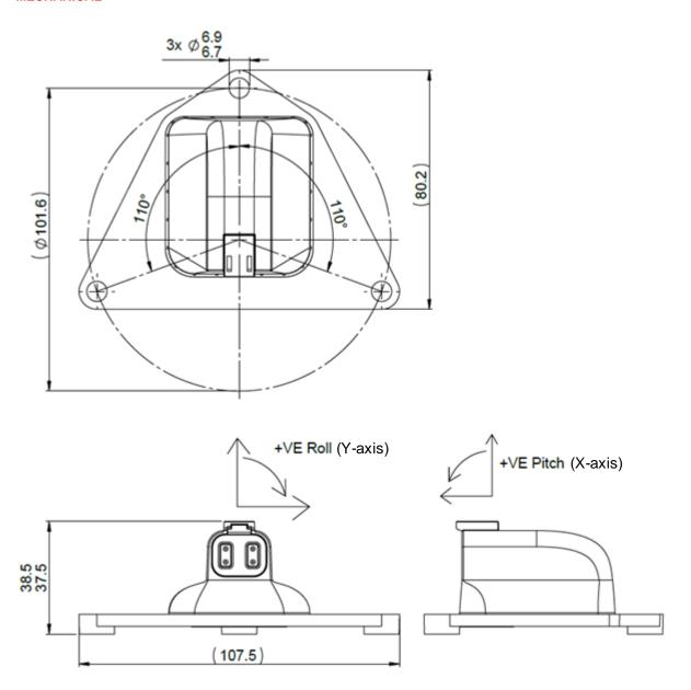
The sensor is to be mounted with M6 or  $\frac{1}{4}$  inch socket head cap screws and washers Recommended tightening torque – 4.5 to 6.5NM Maximum tightening torque – 10Nm
