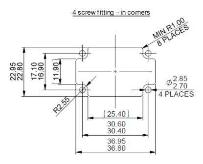
Curtiss-Wright recommend the use of  $4 \times EJOT$  WN1451-K25-12 screws when utilising the 4 corner screw mounting points. The screws should be tightened to 0.3Nm with a minimum panel thickness of 3 mm. For thicker panels the screw length should be increased to suit.
