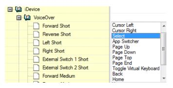
A total of twenty individual R-net commands can be used to control a connected iDevice. This is achieved using programmable Nudge Times which are applied to all four Input Device directions and switch functions. The Nudge Time parameters apply when using Switch Control or VoiceOver, giving a high degree of flexibility to cater for individual users' abilities. Additionally, the Speed Up and Speed Down buttons can be used as further control options.
